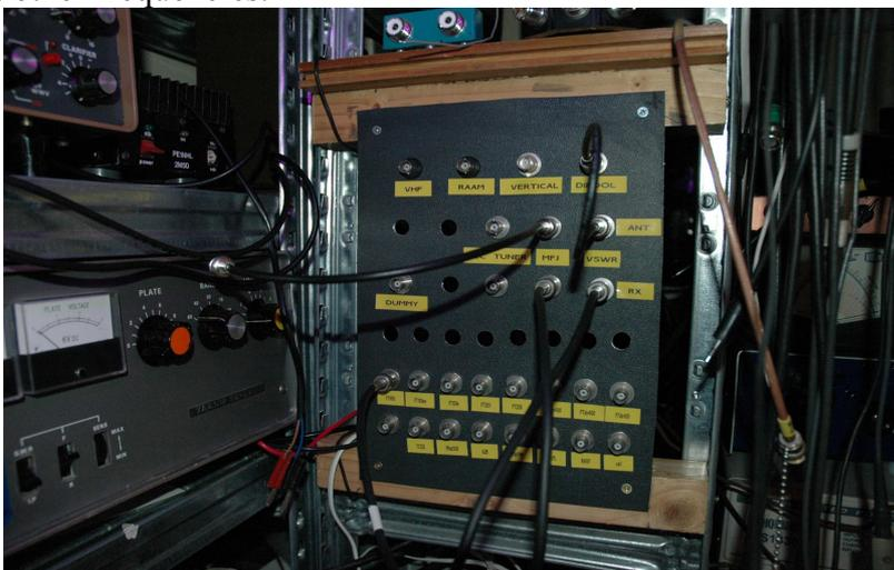
Just to fill up space. My patch panel. Every transceiver has it's own bnc connector. So have the antennas and tuners. When I'm not around all antennas are disconnected in a second.
