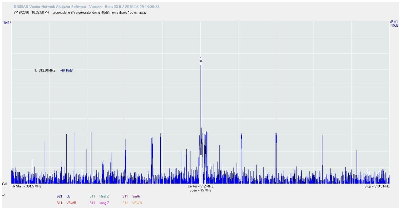
We see the antenna picks up the signal at -40dB. So we lost 30dB between antenna and transmitter. Do not take this values to serious. The VNA can be calibrated to a known source but we are still in the near field and the antenna may have a nice VSWR, but it is not on a good place. Lots of metal around, reflections, me absorbing ect. The function of this picture is to show you the advantage of the SA function.
