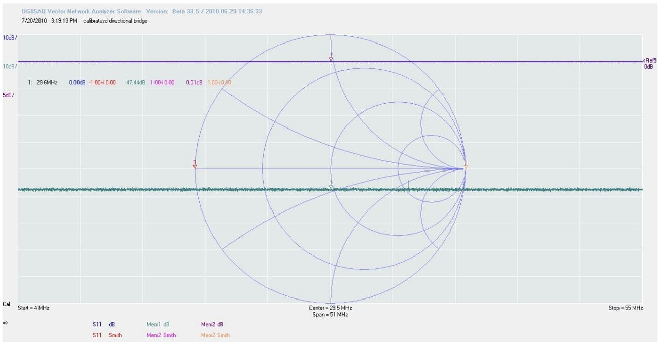
Here, you see a calibrated homemade directional bridge, it has about 35-40 dB directivity upto 501MHz (measured before calibrating).
