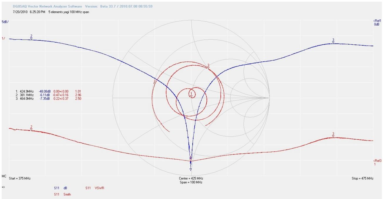
The span in Mmana is max 80MHz so I could not show the whole bandwidth but it was under VSWR 2 from 395 to 510MHz. You see here above this is a rather good simulation. The bandwidth is not that wide as in the simulation but you see, without altering any size I have a working Yagi for 70cm.
