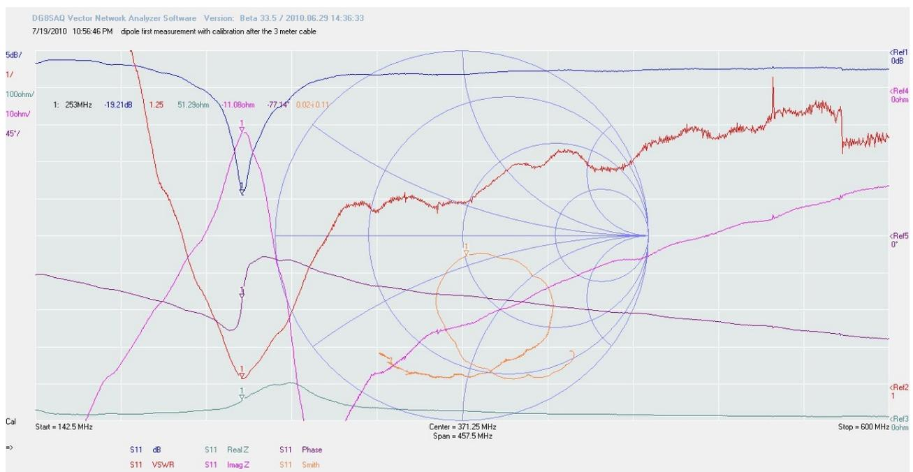
The dipole is now around 250MHz and has a VSWR of 1.25 and that is an impedance of 51-j11 ohm. Lets make that better.
