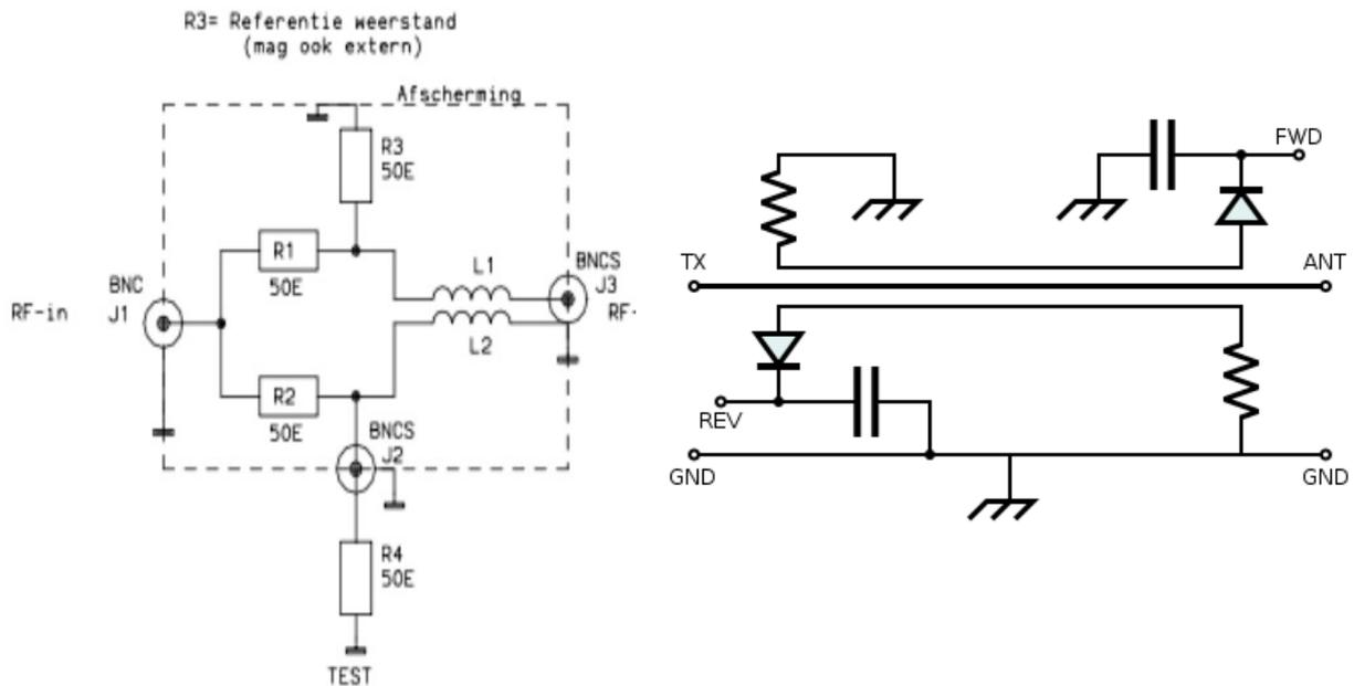
If you use a bridge you can add 20 to 40dB between the bridge and the VNA to protect your VNA. This is not a protection against static but it will take the first blow. However your TX is unprotected. It is possible to add a attenuator there too. But keep in mind you need dynamic range. If this is 90dB and you sacrifice 40dB for the coupler or bridge then you have only 50dB left (most times more then enough)
