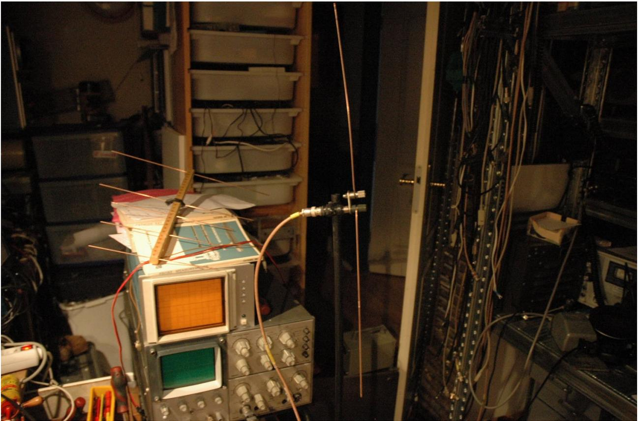
Do not look at the battlefield around it. This dipole is connected on a plastic pole on a small rotor made from a magnetron motor. So I can rotate it.
