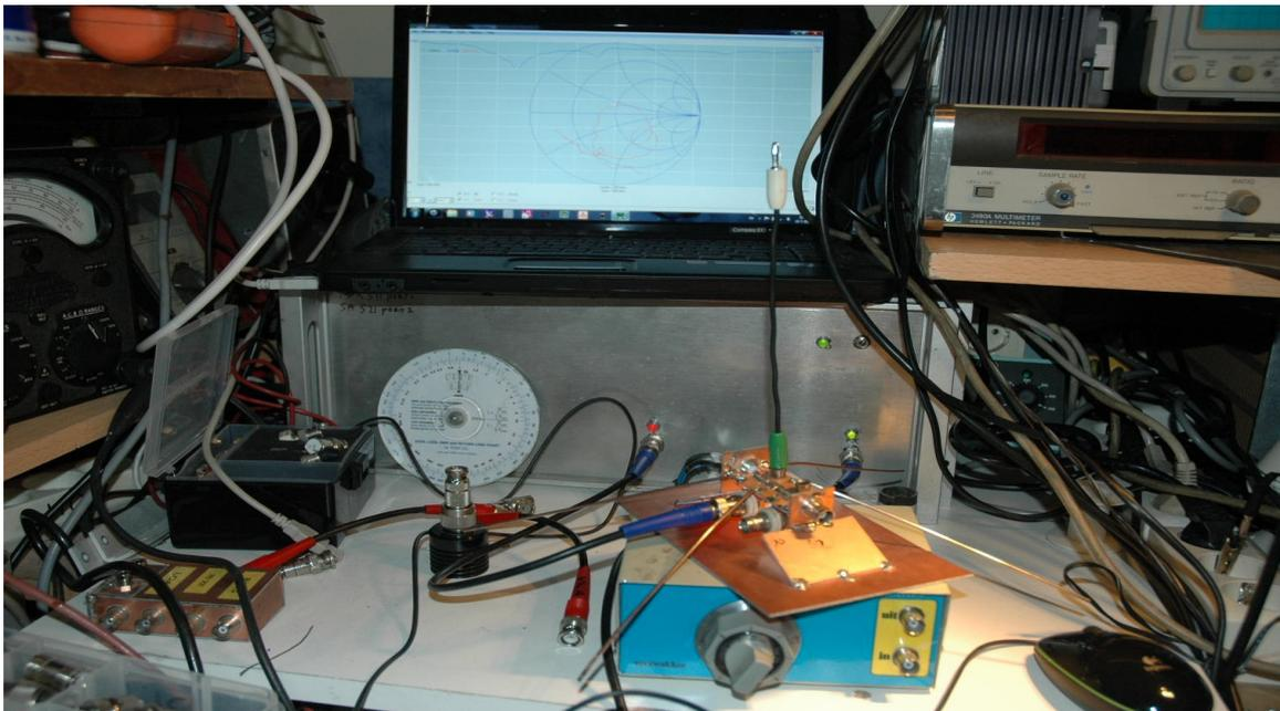
I did this experiments on this nice little DUT-plane antenna. You see, the antenna is just a jump cable with bananas and 4 radials soldered to the DUT holder
