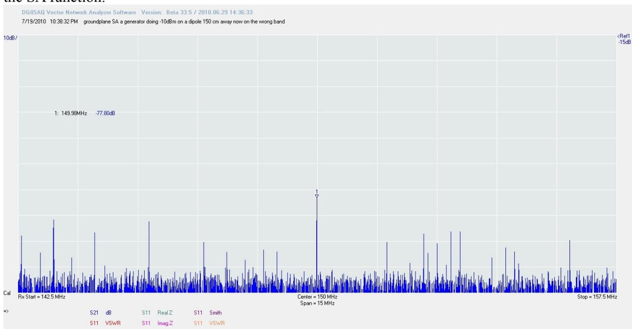
This is the same setup but now I transmit at 150MHz. The signal is now only -77.8dB so you see it works better around the frequency where the return loss is good and a short antenna is rather deaf. It's length is now half of what it should be, the signal received too....
