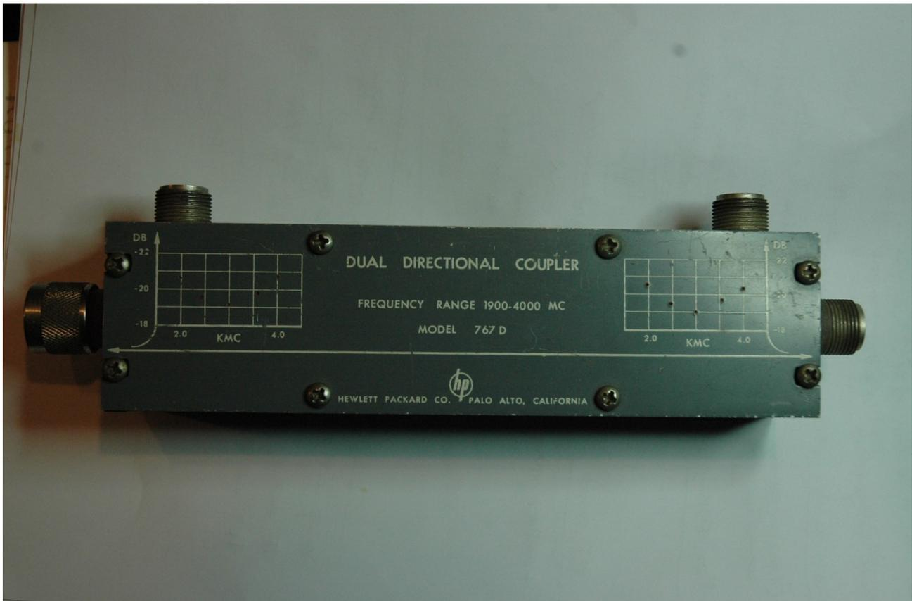
This is a directional coupler from HP. It is to be used between 1.9 and 4GHz but it works good from about 3MHz. I also have one from Ericson that is made for 800 MHz but that does not work well at lower frequencies. The HP is a very robust and well made coupler. The Ericson is more “mass” production.
