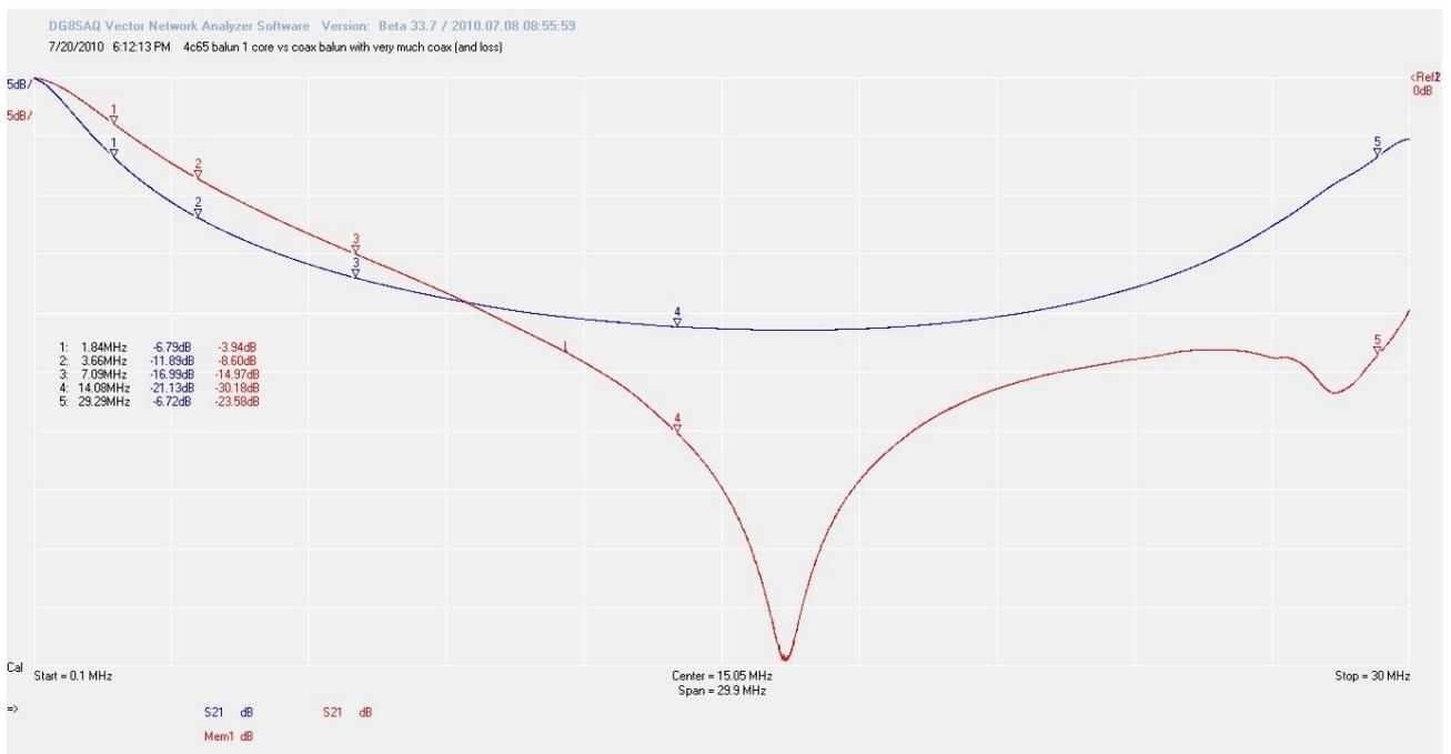
Here you see both of them. The red trace is the ferrite choke on the picture below. It is 8 turns, so not even a meter coax.
