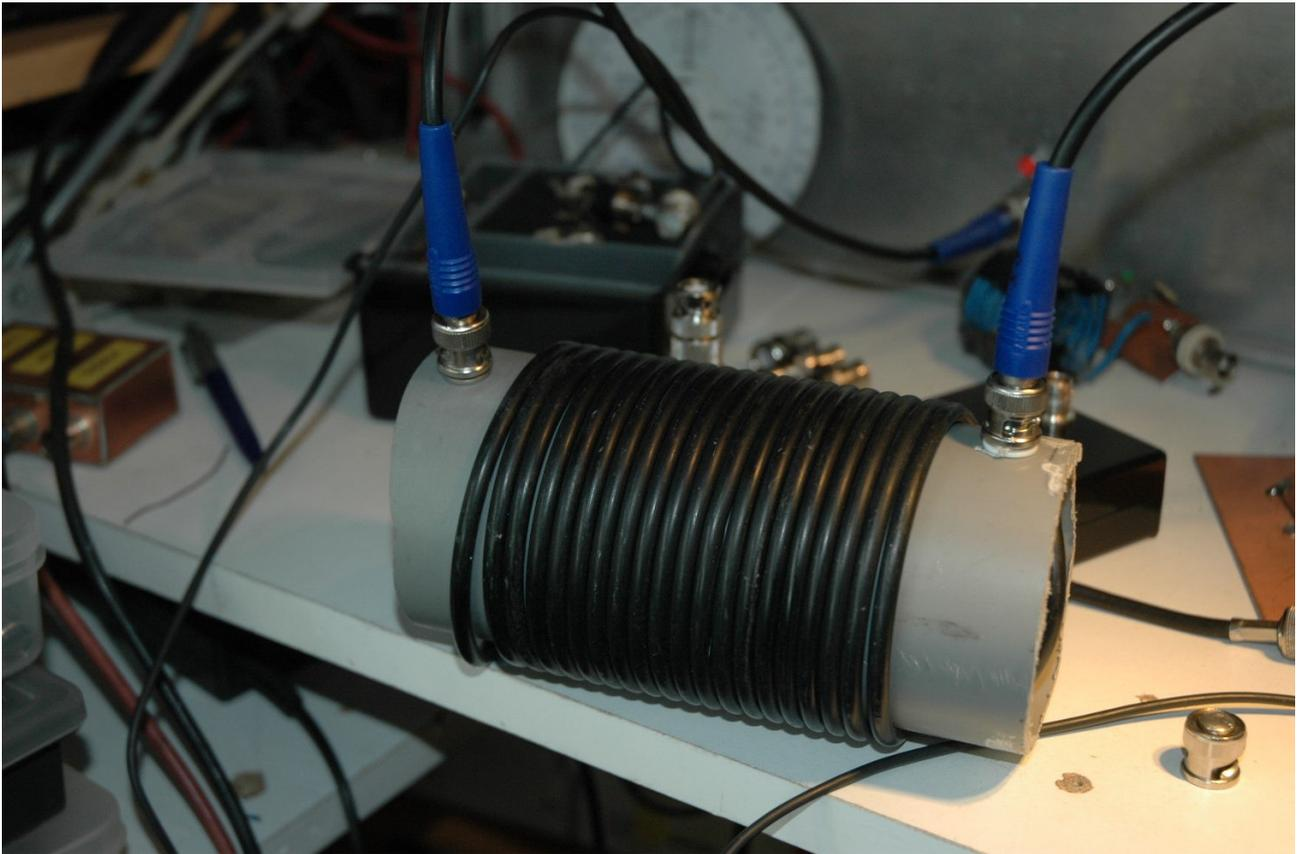
This is the coax one. To measure it I soldered the braiding to the centre of the BNC's so the signal from the VNA has to travel through the formed coil.
