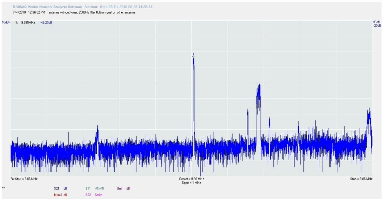
This is how it looks without the tuner. The wanted signal is -43.23dB. That is over 4dB loss. Remember, 3dB is half the power !!!
