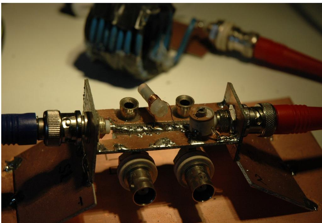
You see a small inductor body with 6 or 7 turns and a ferrite insert. It bridges the gap of the DUT holder.
