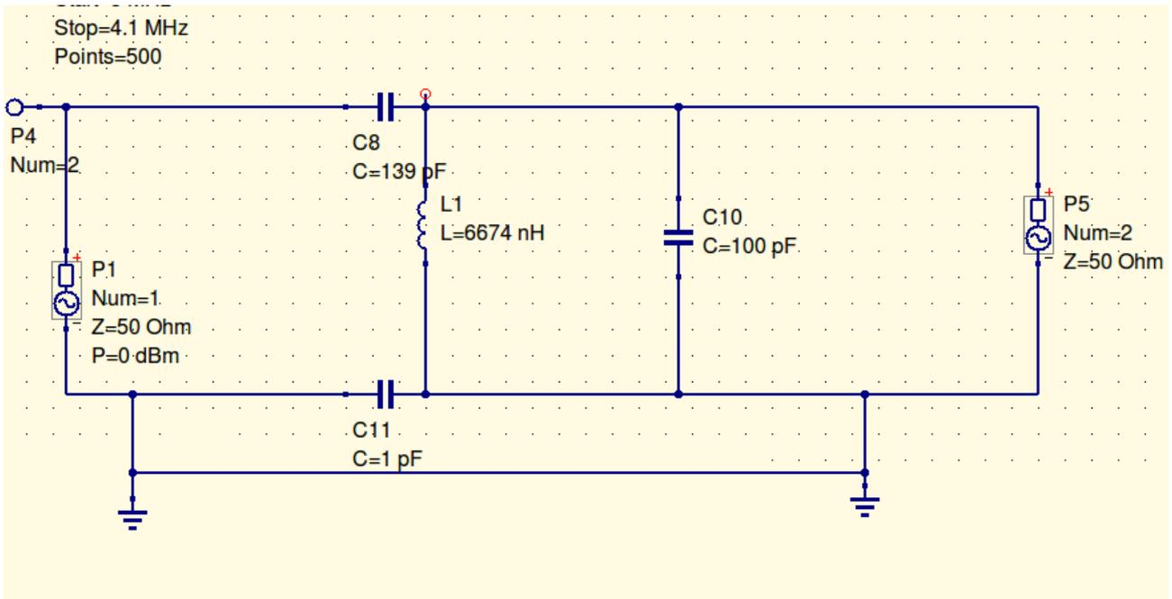
This is what you get if you try a 2 port measurement for a balanced (symmetrical) tuner. You bypass the C11.
