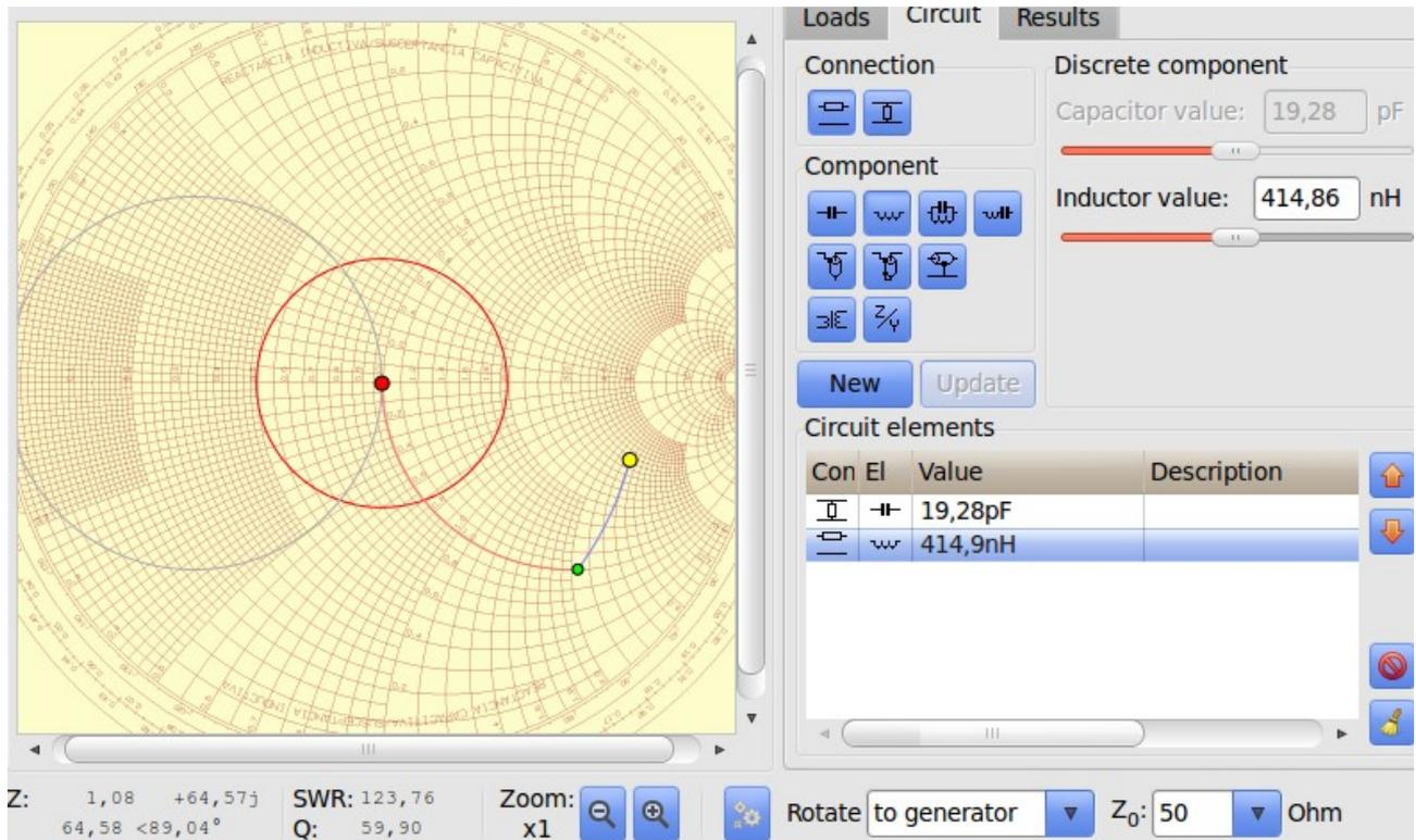
So we need about 20pF and 400nH. But our tuner adds some strays in the construction so probably we need less capacitance and inductance. I just used the mastercall for this test. If you really must know parameters, better calibrate for use at 30-50MHz. The reference plane will be the end of your cable because the DUT holder itself is not important. Your real tuner will also be mounted at a pcb or other construction.
