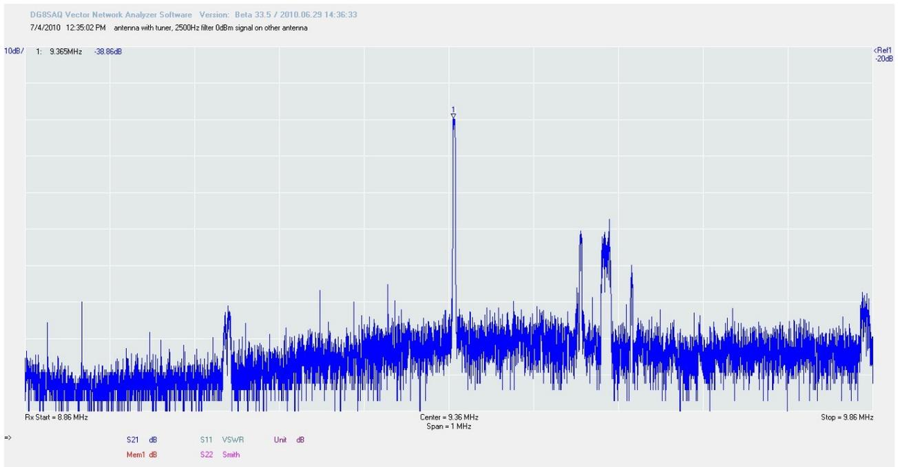
To test the attenuation of a wanted signal I put a 0 dBm signal on my second antenna, a dipole. I changed the span to 1MHz to better see the signal. This is with the tuner in between. -38.86dB
