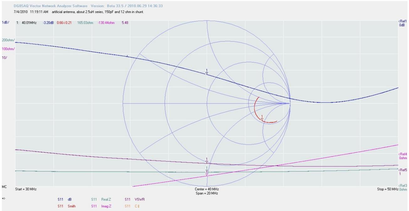
I random took a part of the spectrum where already was a little notch, in this case 30 to 50 MHz. This keeps component values small. The “antenna” has an swr of 5.48 so our tuners has to do an easy job. The antenna is 165-j130 ohm at 40MHz. So our tuner must have a small series inductance and a shunt capacitor at the antenna side. Lets simulate first:
