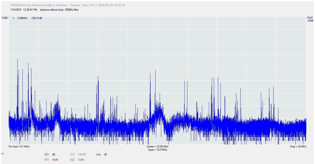
This is the first sweep. I did not use the tuner here. You see signals over the whole sweep. Noise level is raised to -100dB. Lets look at the effect of the tuner.
