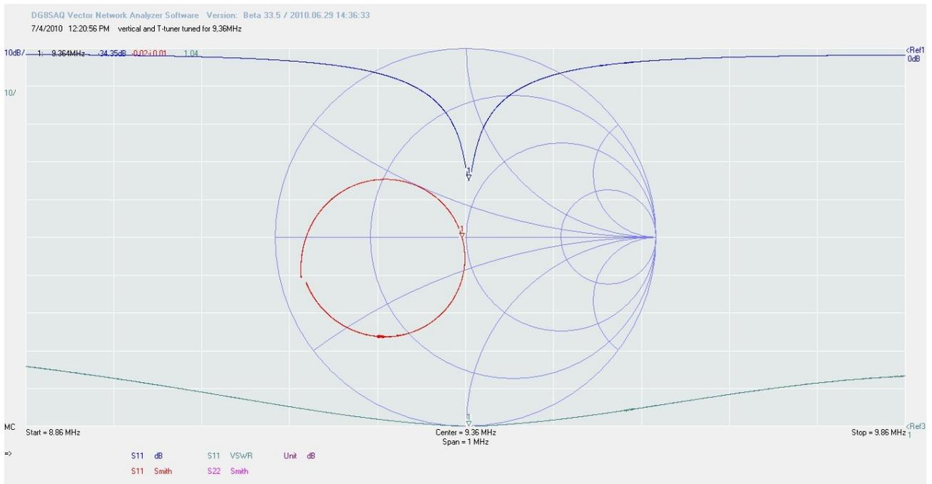
It was hot and I'm lazy, so a random tuning gave this resonance. But also because the vertical is resonant at almost all higher HAM bands above 40m so I needed an impedance that was hard work for the tuner. Now the tuner is set we are going to test it the same way.
