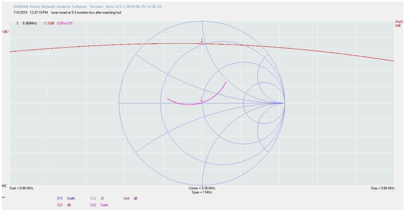
The tuner measured like before (VNA on in and output) and using the matching tool gives us a loss of 1.33dB.
