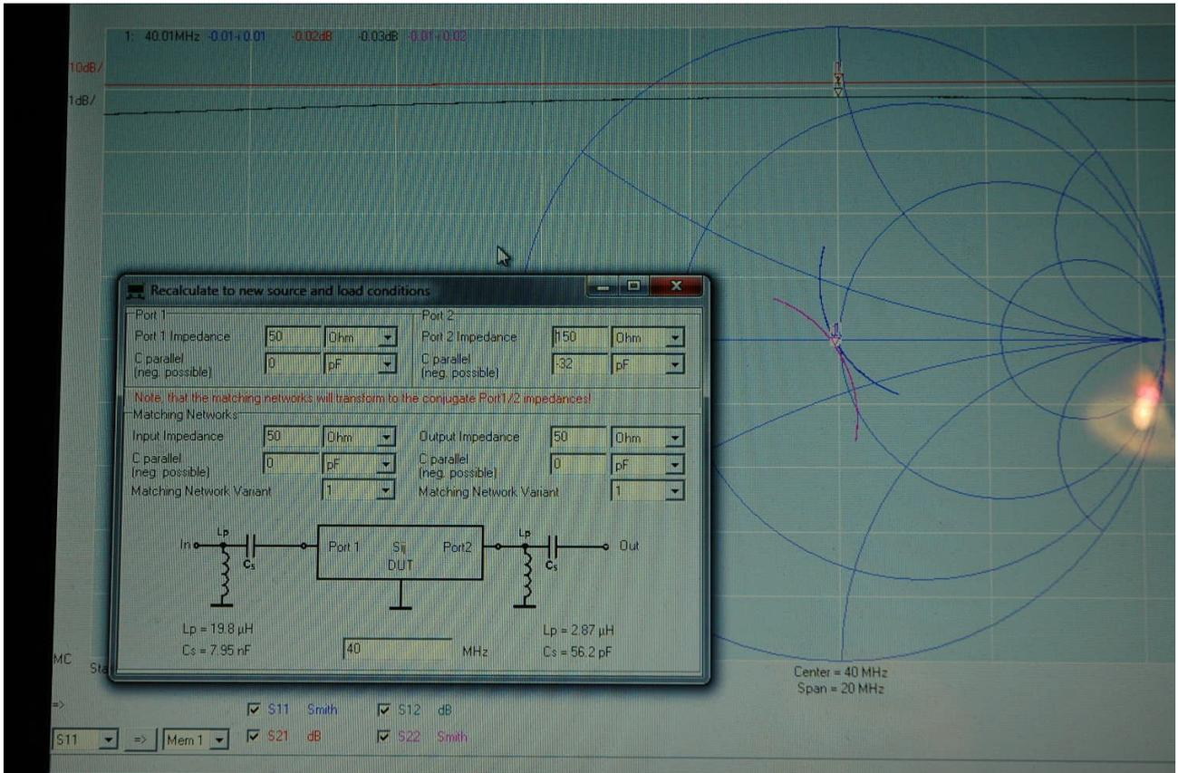
You can read the value of S21 in next screendump. This one is made the right way (the picture was done later to show the matching tool) and you see the tuner has a 0.17dB transmission loss. You can make a check by connecting the cables without the tuner and do a S21 sweep. The loss must be almost 0dB. In this case, if we would transmit 100W, the loss in the tuner would be around 4W. I bat you lose more in the cable towards your antenna.
