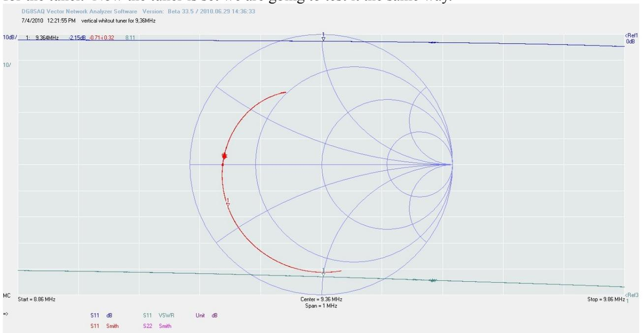
This is how the vertical looked without the tuner. A VSWR of 8. So not extreme but more then an internal tuner is capable for.
