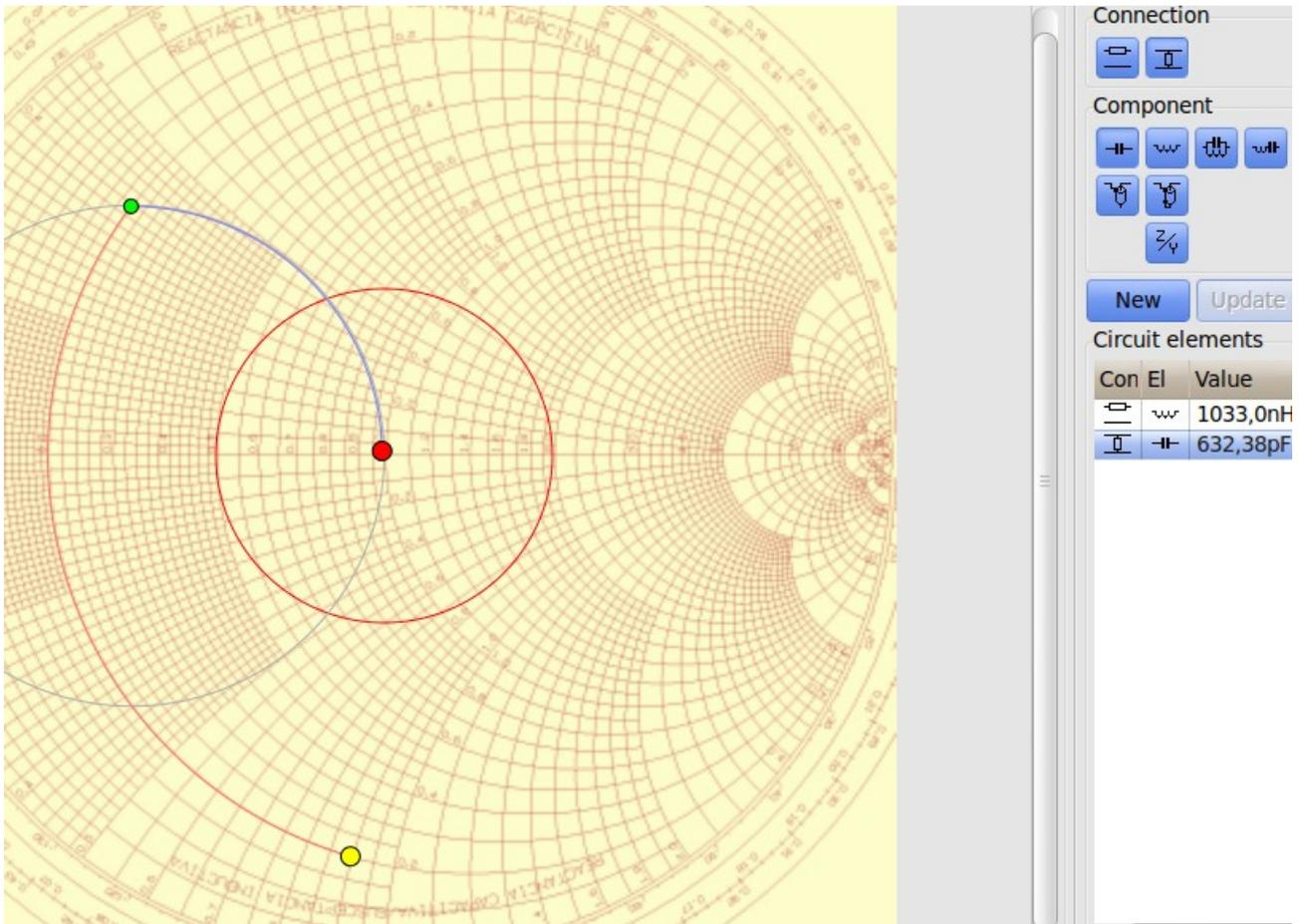
Yellow is again the load. The blue line the shunt capacitor, again travelling over an admittance circle, the red line is the inductor travelling over an impedance circle. The inductor has almost the same value, this is because the inductor only changes the imaginary part. It does not change impedance. The shunt capacitor changes the impedance. That's why it changes in value and in location.
