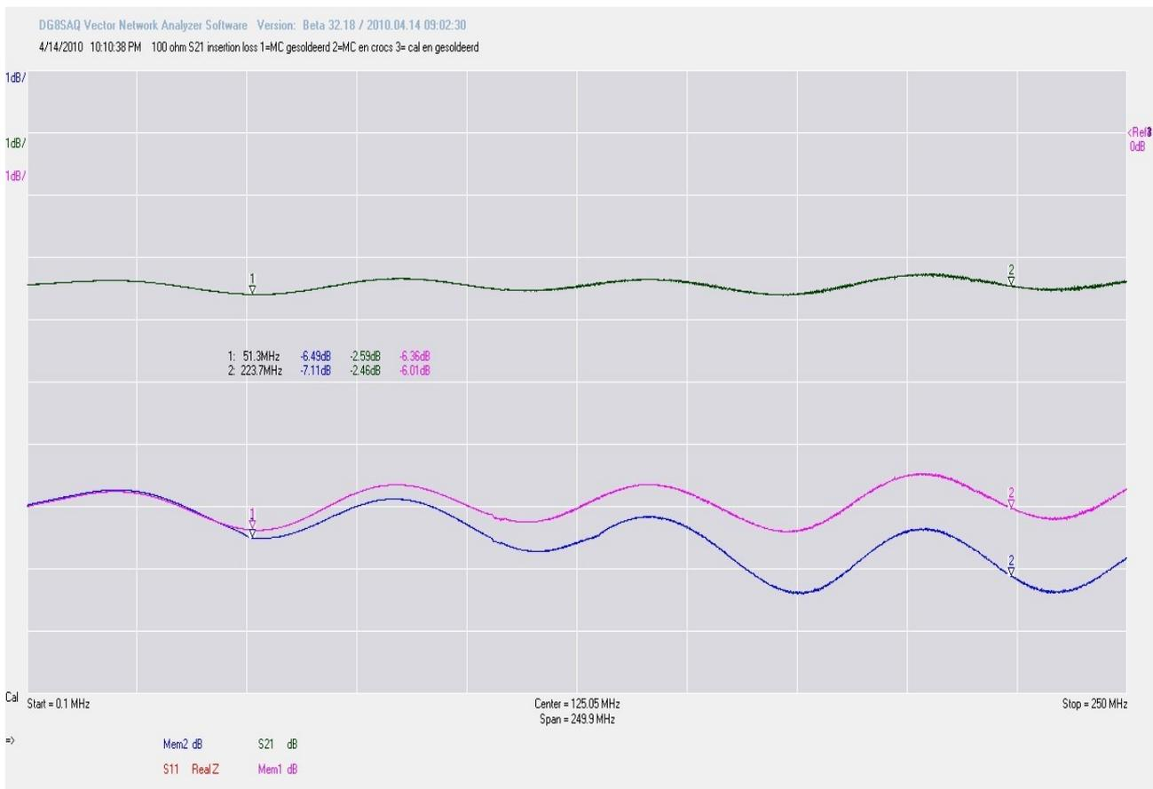
The purple trace mem1 gives the sweep using the master cal and the resistor between the crocs, mem2,
