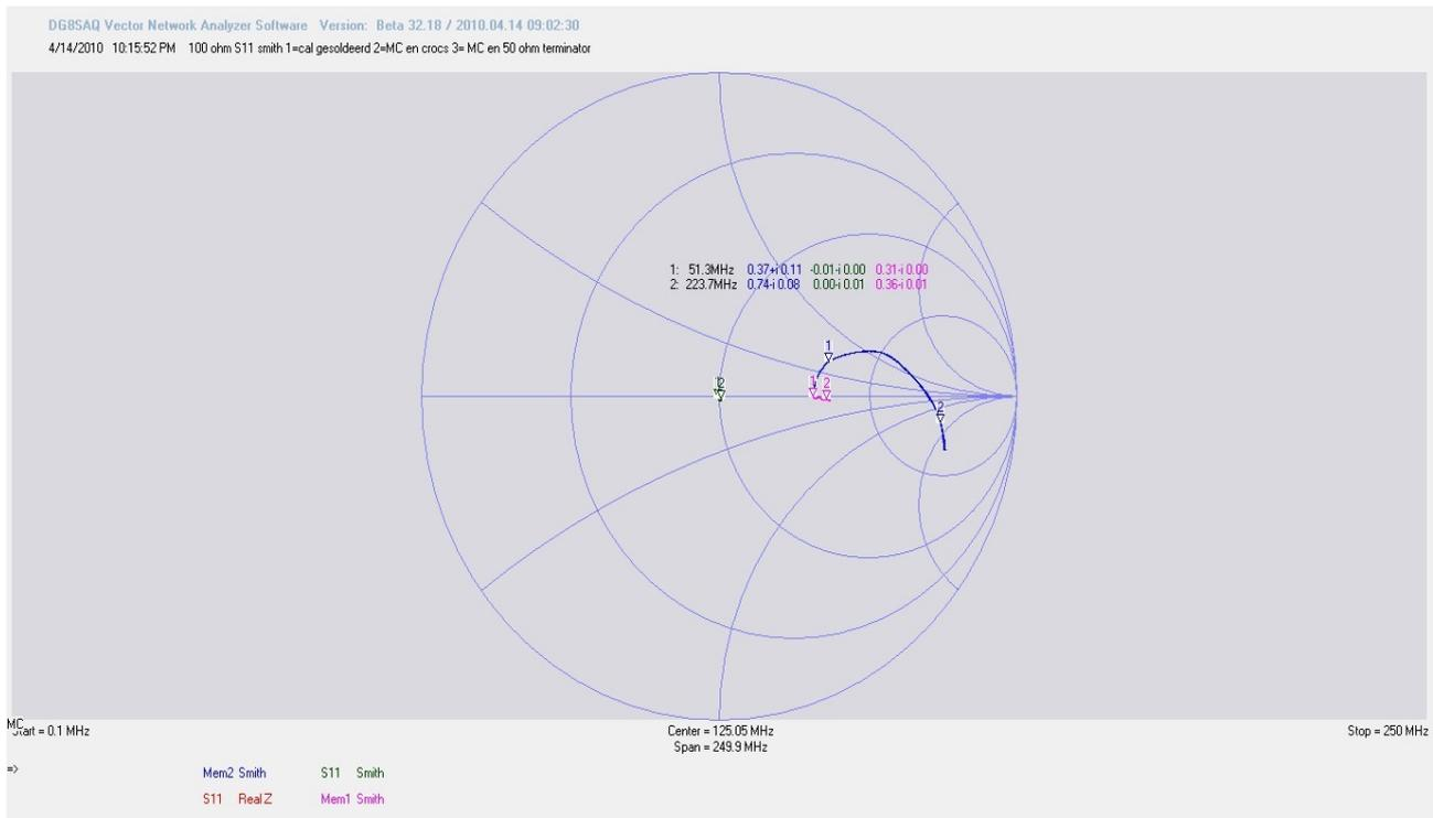
The **blue** line is our resistor with the long wires in the crococlips You see at 52MHz the wires and poiles of the crocs form an inductance. Remember, this is the sum. There is also a capacitance involved from the two crocs next to each other but the inductance is much bigger. You see that as the frequency goes up. The line passes the centre line, there the capacitance is as big as the inductance, the sum is zero. We call this resonance. ( $+20j + -20j = \text{zero}$ )
