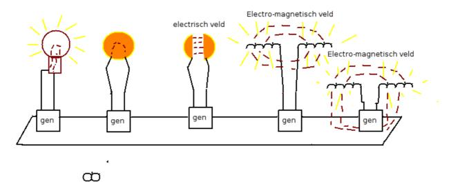
So here we have an antenna. The different versions and forms all have to do with impedance matching, direction of radiation, gain and polarisation. This is why it then get so complicated, but remember all those antennas still have the same basics.
