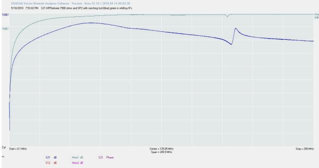
This time the capacitor is between port 1 and 2 and the coil is to earth. If we measure it without knowing the impedance (in this case the two resistors) the filter looks like the blue trace. This does not make you jump up in joy. Attenuation over the whole range.
