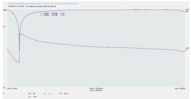
Just an in between. If we build the circuit and parts well, we get the picture above. This is up to 250MHz. So no other resonances like the picture below. There you see a compare between the two capacitors over a 250MHz sweep. You see the effect of the Q of the variable capacitor. The bandwidth is a bit more narrow. You also see the effects from wires to the capacitor and coil.
