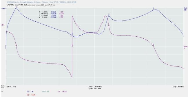
We see at 14,8Mhz the resonance. This indicated that the influence of the loading is bigger. The resonance frequency went down. We also see the phase jump. We see more resonances. At 93MHz we see a parallel resonance. But we did not use a parallel circuit so here we are looking at parasitic behaviour. Dangerous because this can cause a an amplifier to start oscillating at 93MHz.
