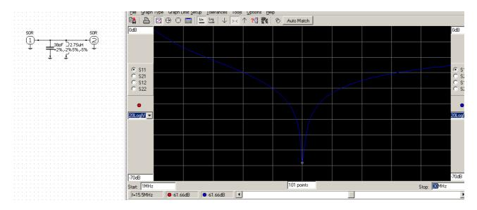
Nice isn't it. We see a resonance at 15,5Mhz. You also see a strange thing. The signal behaves not symmetrical. The first half is done by the inductor, the second half is merely the work of the capacitor and you see, they do not have the symmetrical slope. If you look in chapters 2 and 3 you see at first a fast rise/fall and and later a slowly changing curve.
