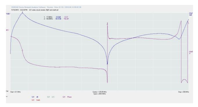
This is also a series circuit, but now with an other coil. This shows a really big parallel resonance. This is not a good build circuit. What have I done ? I had the coil almost flat at the ground surface. So I introduced a capacitor parallel at the coil.
