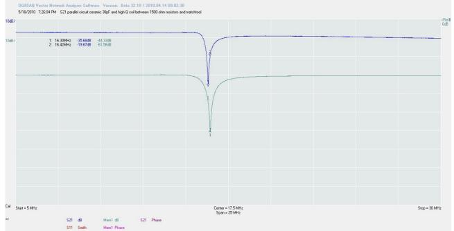
First look at the green trace in Mem1. It is attenuated by the resistors but you see it gives a much sharper dip as the pictures before. But we want to correct for the mismatch so after doing a SP2 2 port measurement to memory we open the tool menu and use the matchingtool. Type 1500 ohm at
